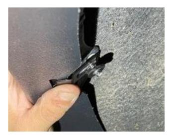
**STEP 5-1:** Using the factory screws that were previously removed, attach the clips to corresponding existing holes (X4) in upper inner wheel well. Do not fully tighten screws at this stage.
