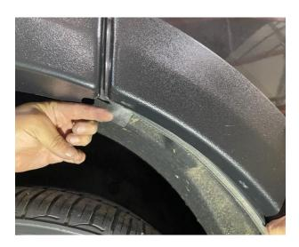
**STEP 24:** Place fender flare up against vehicle for best fit by aligning the end of fender flare with the doors edge as shown above. Align abrasion resistant tape with the (3) slots in fender flare. Remove fender flare.
