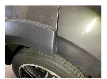
**STEP 18:** Re-apply fender flare to vehicle in best fit position.
