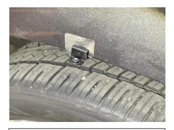
**STEP 17:** Slide push-on clip over the abrasion resistant tape in alignment of the slot in the fender flare
