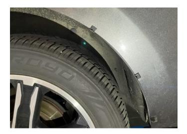
**STEP 25:** Slide push-on clip (X3) over the abrasion resistant tape in alignment of the slot in the fender flare
