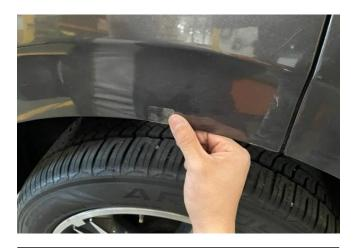
STEP 16: Place tape on to the painted surface of the vehicle as shown above.
