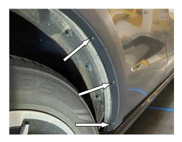
**STEP 26:** Apply pressure to the fender flare to create tension against the vehicle and begin to fasten all (3) mounting points as shown above. If slots are misaligned, you may need to adjust tape and clips accordingly when tightening.
