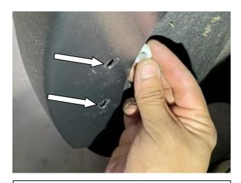
**STEP 19:** Place 5mm spacer behind the (2) slotted holes of the fender flare and begin to loosely install using the long screws supplied in the hardware kit.
