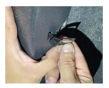
**STEP 5:** Secure attachment clips (X4) by sliding clip into Fender Flare slot. As shown above.
