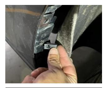
**STEP 12:** Install U-nut over existing hole of the hard plastic, not the tab of the painted surface.
