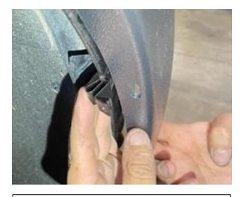
**STEP 6:** Slide push-on clip over the abrasion resistant tape in alignment of the slot in the fender flare. Use the small screws supplied in hardware kit to fasten.
