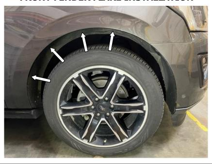
STEP 2: Using a 5.5mm socket / wrench remove factory screw locations (X4) where noted above and retain for re-install. Clean the body areas where the Fender Flares will contact the vehicle surface. Ensure fenders are dry prior to install.
