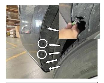
**STEP 11:** Remove the (5) push in fasteners for ease of installing the (2) U-Nuts. The U-nuts will be installed in the positions circled above.
