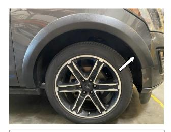
STEP 3: Hold Fender Flare on the vehicle in the position of best fit. Note where above marked slot is in the Fender Flare.
